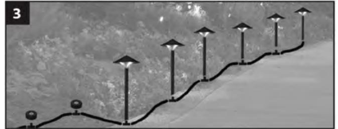
3. Run all wires from the power source locations to the light. on top of soil, remember to leave slack. If using separate circuits with independent dimmers, we recommend grouping lights by type.
