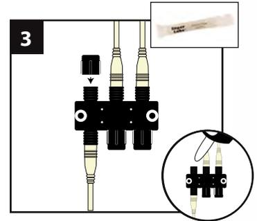
2. Attach male lead from lights to female connections on splitter. Attach male to male connection wires in between each splitter. Continue until all wiring from lights are attached to splitters and connector wires are attached in between splitters. If lights are spaced several feet apart use T-splitters.
