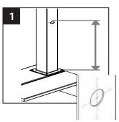
**NOTE:** If deck boards are not installed yet place an appropriate deck width spacer board to ensure post sleeve is at correct height.
