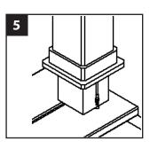
5. Add a small silicone bead around the back of the light.
