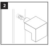
3. Measure and mark the location of the wire pass through hole in the deck board based on the wood post and sleeve. If an aluminum rail is used measure based on the hole in the bottom of the post. use a 1/2" bit to drill the hole for the wire pass through.
