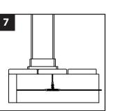
**NOTE:** If railing has already been installed, lead wires will need to be fished through the post sleeve to reach the desired location for the deck rail light. In some cases if the provided lead wire does not fit (due to connector size), the wire connectors can be cut off and wire nuts can be used. Test lights with the power on. If lights wired with this method do not function, switch the connector wires.
