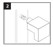
4. Feed the wire from the light through the hole in the post sleeve. Feed the bottom of the post sleeve though the post sleeve skirt. Carefully while holding the wire out of the way at the bottom slide the post sleeve and skirt assembly over the wooden post.
