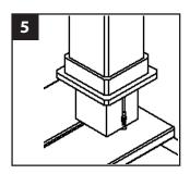
8. Connect the pigtail to the cable and push into post. Fasten bracket to post with screws.
