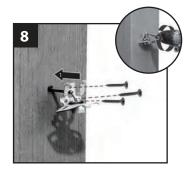
6. Feed wire through deck board. Secure aluminum post to deck board with provided anchor bolts.
