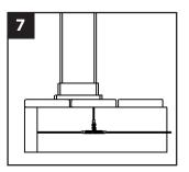
**NOTE:** If railing has already been installed, lead wires will need to be fished through the post sleeve to reach the desired location for the deck rail light. In some cases if the provided lead wire does not fit (due to connector size), the wire connectors can be cut off and wire nuts can be used. Test lights with the power on. If lights wired with this method do not function, switch the connector wires.
