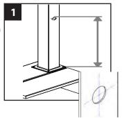
3. Measure and mark the location of the wire pass through hole in the deck board based on the wood post and sleeve. If an aluminum rail is used measure based on the hole in the bottom of the post. use a 3/8" bit to drill the hole for the wire passthrough.
